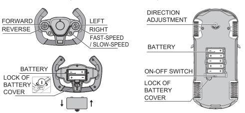
Function: forward, reverse, turn left, turn right, headlight,rear light,fast/slow speed change, topspeed overtaking, slow-speed driving, open/close doors manually default slow-speed when boot, press to shift between fast-speed and slow-speed, press the Forward or Reverse button, indicator on remote control will flash when in fast-speed, and keep on when in slow-speed.
